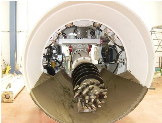
Road header in open shield
