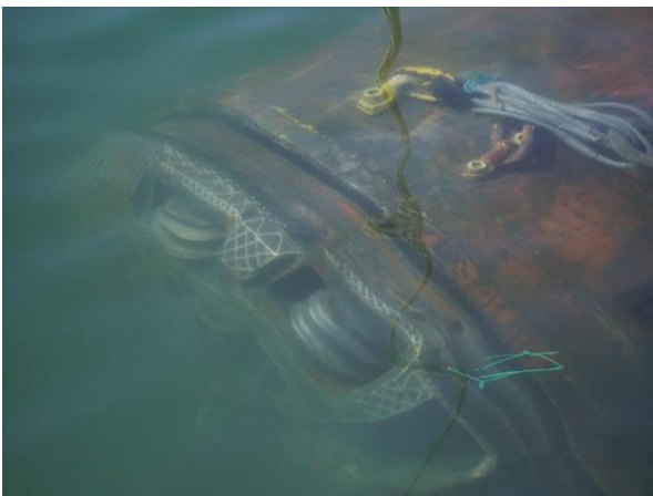
Hydro shield machine in port after an outfall drive
